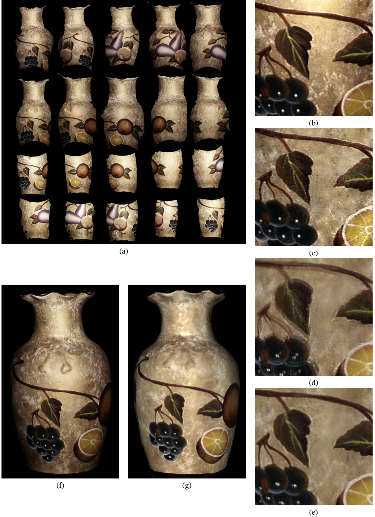
Fig. 10. The vase dataset. (a) The twenty scans used to reconstruct the vase. (b) Intensity image captured by the scanner. (c) Computed albedo map. (d) Reconstructed albedo without image-based registration. (e) Same as (d) with image-based registration. (f) Photograph of the vase. (g) Rendering of a computer model of the vase reconstructed from the twenty scans.
